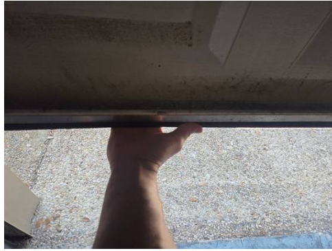
Garage door opener reversed direction properly when resistance was applied during testing.
